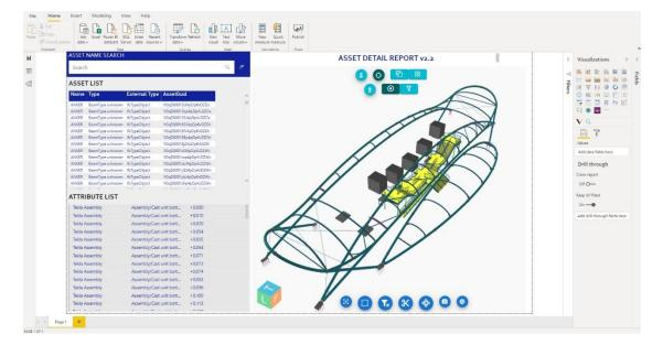
By selecting one or more assets in the table the corresponding element is highlighted in the model and the attribute list shows the relative attributes. The custom visual functionalities allow for an easy identification of object both from the list and by clicking on the model.
