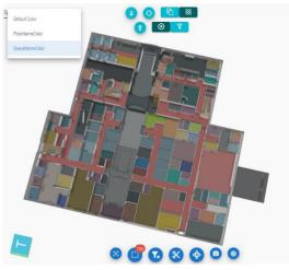
Vcad allows for different types of coloring depending on type, name, room collocation, etc. indistinctly for assets or spaces.
