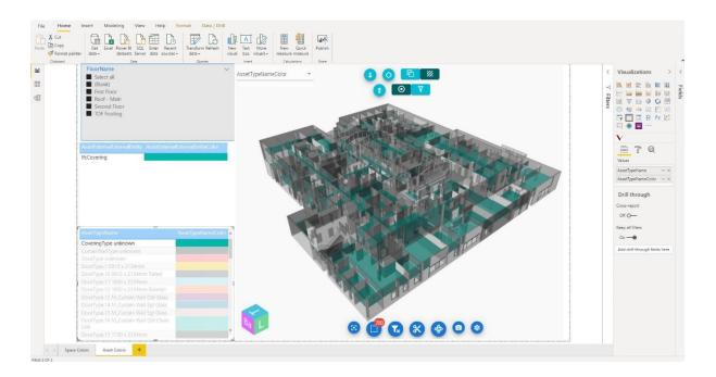
As for the spaces, the Vcad custom visual allows the coloring of assets based on the type or name. The different coloring combined with Vcad's functionalities allow for easy identification of the elements of the .ifc file.
