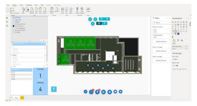
Depending on the selection in the "Floor Name" list, the model will be filtered by that floor and highlight the spaces within it. The description and name list allow the user to filter the desired spaces.
