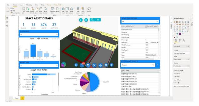
The template contains the information of the structure of the model, starting with the number of assets and their attributes. The filters defined concern the floors, the assets per floor or the assets per type of space.
