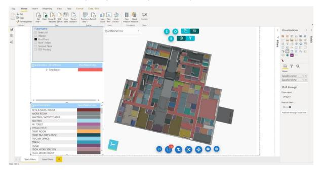
The user may select a floor and filter the spaces by name and intended use. The Vcad custom visual allows for easy identification of the desired space thanks to the use of a specific color.
